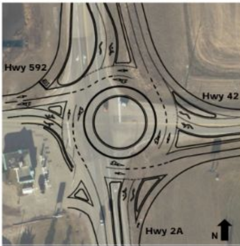
Figure 1. The new roundabout configuration
